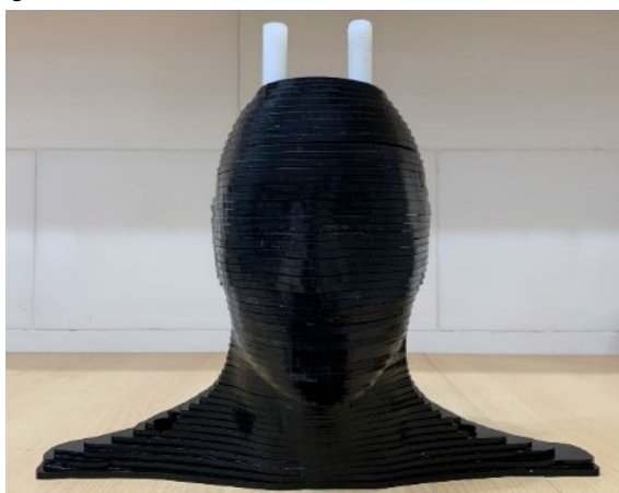
Figure 1. A general view of the assembled cost-effective head and neck anthropomorphic phantom. The phantom is constructed from stacked 5 mm thick laser-cut plates of plexiglass (soft tissue-equivalent) and polytetrafluoroethylene (PTFE, bone-equivalent), secured with alignment rods.
